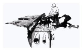
9. Complete placement of backfill behind forms. Place layer of flattened empty bags on top of the GILSULATE® 500xR envelope. Hand place 4" to 6" of soil (no stones) on top of empty bags to protect from damage. Complete backfilling to grade level as soon as possible. Mechanical compaction of backfill is desired and follows good engineering and construction practice.
