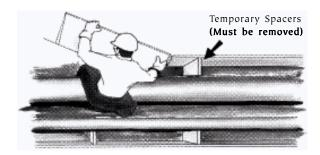
3. Side forms are recommended. Side forms cut from gypsum board and left in place are less expensive and easy to use. Forms are held away from pipes by temporary spacers which must be removed. Side forms left in place must not extend above the finished compacted level of the insulation envelope. Forming is always the preferred technique.
