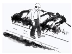
8. Walk on consolidated **GILSULATE® 500**xR envelope to ensure use density, footprints less than 1" deep are required.
