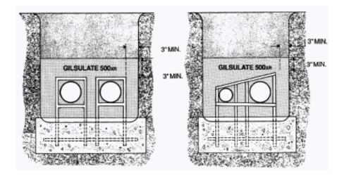
Note: Concrete and metal surfaces where in contact with GILSULATE® 500xR shall be coated with bitumastic (see note on page 8).
