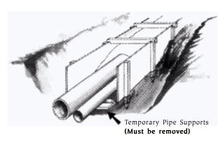
Precut gypsum board with attached spacers on the exterior may be driven into place quickly. Horizontal spacer is used to determine envelope width. Backfill behind the forms to pipe height. Leave forming in place. **Calculate volume required per lineal foot of trench.** One bag equals 1 cu. ft. at use density (following consolidation).
