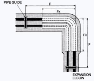
Dimensions A, B and C shall be the dimensions A, B, and C (from Table No. 1) x1.5.
