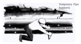
2. Grade and compact trench under pipes leaving required space for specified thickness of **GILSULATE® 500xr**. Clean dirt off pipes.
