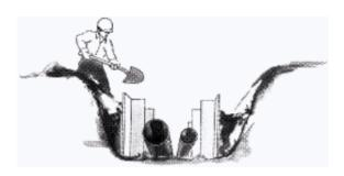
**4.** Check all measurements for correct insulation coverage. These are given in the plans and specifications or may be found in the GII "Design & Installation Manual." Backfill behind forms to pipe height.
