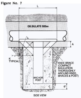
Note: Concrete and metal surfaces where in contact with GILSULATE 500xR shall be coated with bitumastic. (See note on page 8)
