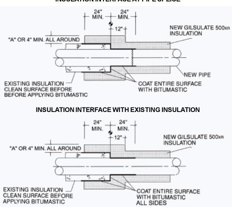
Interface of existing insulation system retrofitted with **GILSULATE®** 500xR. Contact Gilsulate International, Inc. for details specific to the interface between the new **GILSULATE®** 500xR and the existing insulation system.
