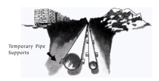
Excavate trench as required for piping and insulation and preferably pile all backfill on one side. Install pipes with required guides, supports and anchors. Perform pressure testing. Locate pallets of GILSULATE® 500xR on the side opposite the backfill.
